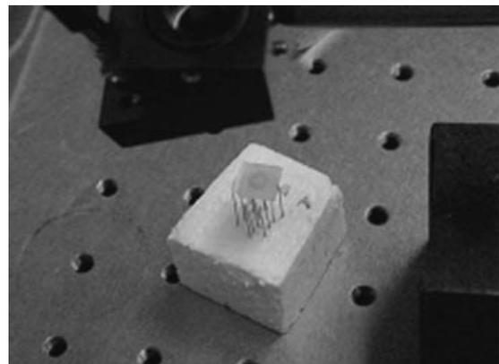
Fig. 2. Digital photograph of typical specimen placement on stainless steel taxidermy pins.
