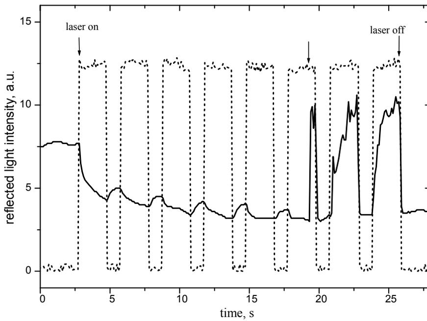
Fig...4.. Typical time dependence of the optical signal of the feedback control system in the course of laser irradiation of spine disc.
